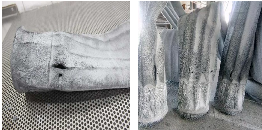
Figure 6. Abrasion damage of filter bag.
